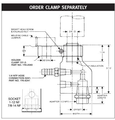
To determine distance adapter sticks out from holder, deduct 1/2-in from length of adapter selected. Water tubes 1/2-in. longer than adapter will install approximately flush with adapter face.
